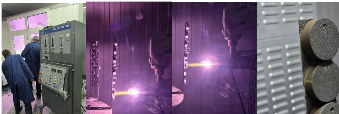
Figure Stages from APS of complex ceramic powders
